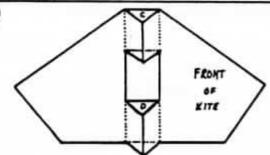
Fold on centerline. Tape sections "C" and "D" to back to form two triangular box sections, top and bottom.
