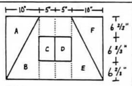
Cut on solid lines; fold on dotted lines. Note: 6 + 2/3" equals 170 mm.
