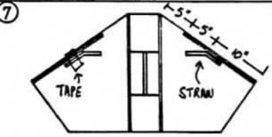
Bend piece of straw in half. Tape along side wing spar, leaving one half of straw free to move.
