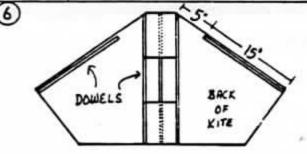
Glue 16" sticks to leading edge of wings. Glue 2 20" sticks to back of triangular box. Glue 1 20" stick inside leading edge of box.
